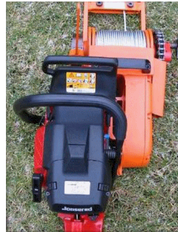
LEWIS WINCH WITH POWERHEAD ATTACHED
